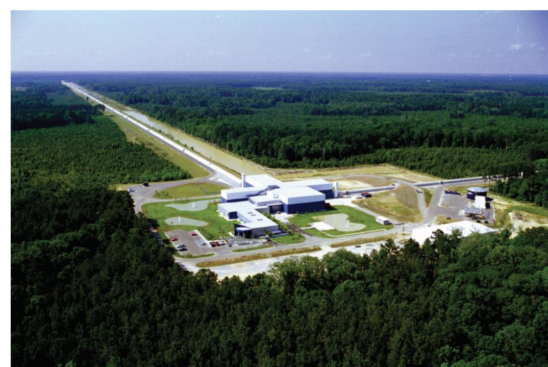
LIGO is a Michelson interferometer that detects gravitational waves by precisely estimating the relative laser phase shifts
